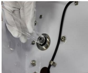
**Step 7:** Hand-screw End Nut on the Reactor Chamber.
