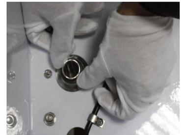
**Step 8:** Screw the nuts tightly on the reactor chamber. Firm hand tightness is sufficient. Tools should not be used so as to avoid damaging the quartz sleeve
