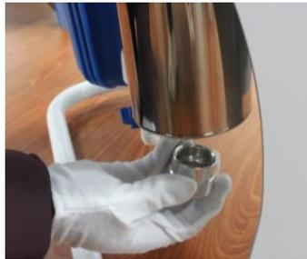
**Step 6:** Insert the Quartz Tube into the Reactor Chamber.
