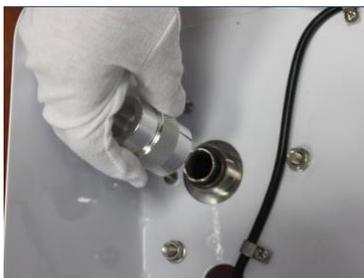
**Step 9:** Carefully insert the UV Lamp into the Quartz tube
