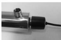
**Step 3:** Remove both Open and Closed End Nut from Reactor Chamber.
