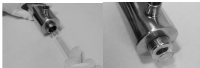
**Step 8:** Hand-screw Open End Nut on the Reactor Chamber (open end of Quartz Tube). To protect the O-ring, do not over tighten.
