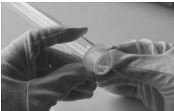
**Step 6:** Insert the quartz sleeve into the Reactor Chamber.
