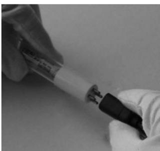
**Step 9:** Very carefully insert the quartz sleeve through the end nut onto the UV lamp
